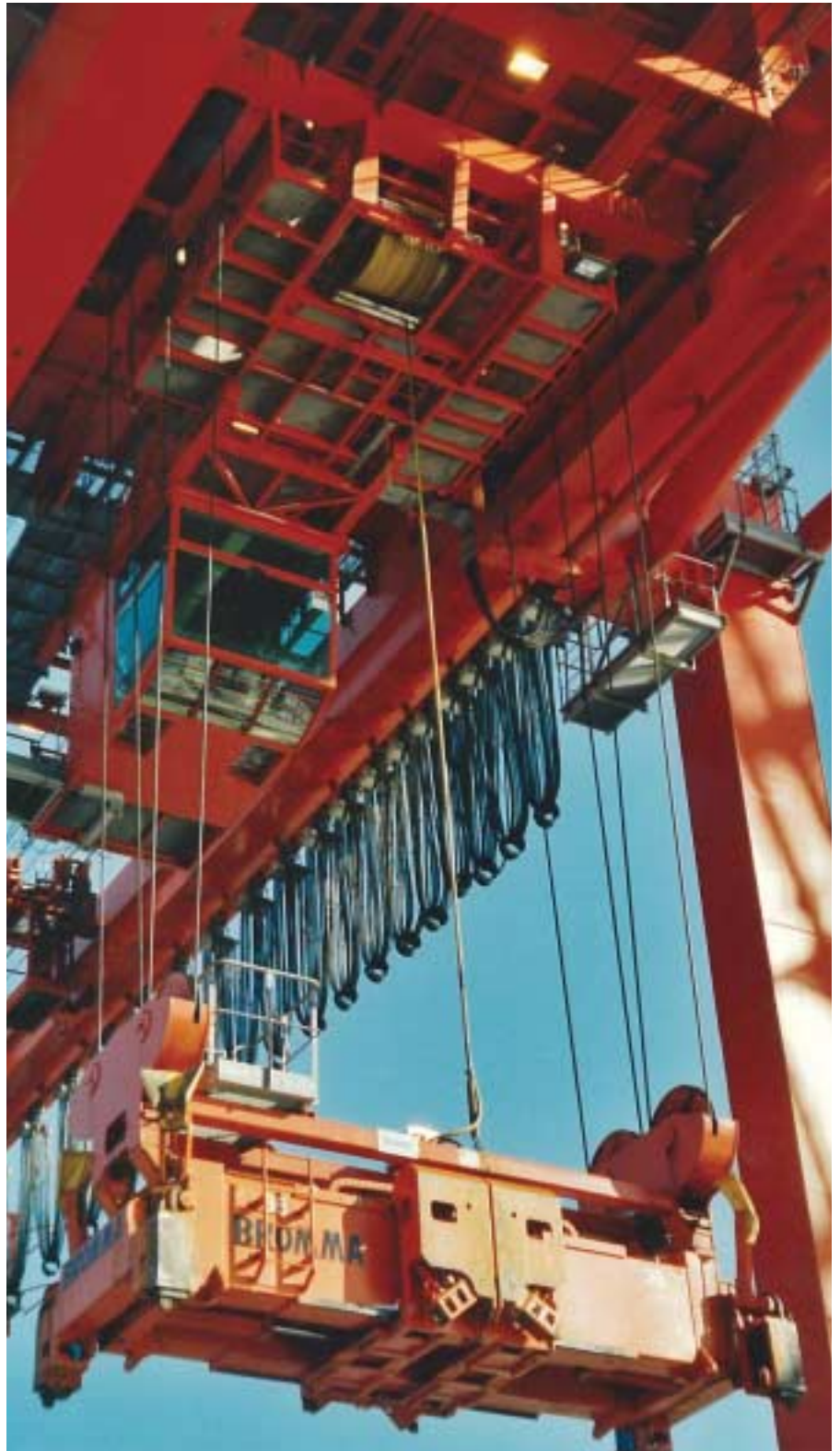
A Cavotec Specimas Spreader Reel in action.
